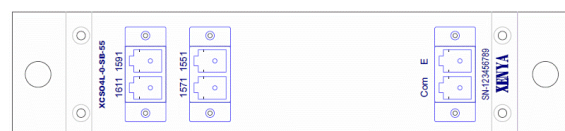
Figure 5 XCSO4L-0-SB-55_A2 - Single fiber Single side 4 wavelengths CWDM OADM version B
