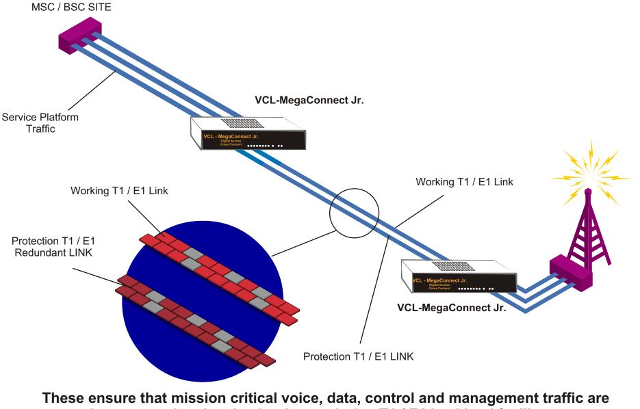
properly supported and maintained even during T1 / E1 backhaul facility outages. When the working link fails, the protection link becomes active.
