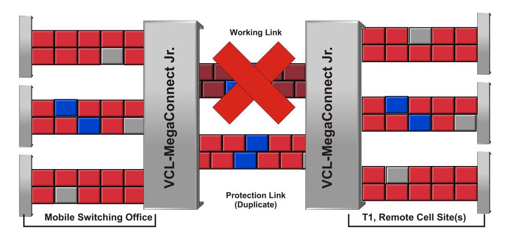
In the event of a failed or degraded T1 / E1 link, the traffic is automatically transfered from the previously working link to the duplicate protection link in accordance with the pre determined operating parameter programmed by the network operator.
