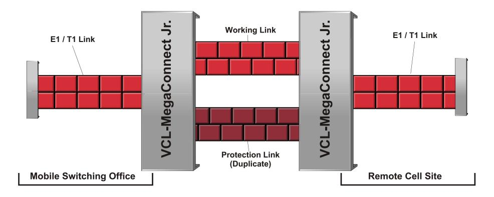
During normal Operation, VCL-MegaConnect-Jr sends duplicate traffic across both the working and dedicated protection E1 / T1 facilities while continuously maintaining the performance of both links to determine which link shall be utilized.
