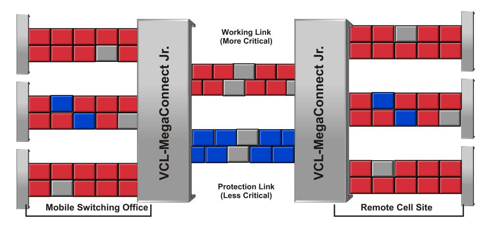
During normal Operation, VCL-MegaConnect-Jr APS passes independently traffic across both the working and protection E1 / T1 facilities while continuously maintaining the performance of both links to determine which to utilize for critical traffic
