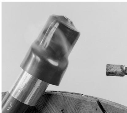
Simply heat the cap until it has shrunk tightly over the cable end
