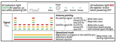
If the terminal does not have a GPS fix, leave the terminal to acquire a GPS fix. This may take a few minutes. While the interface unit is searching for a GPS fix, the Signal indicator flashes green and red alternately and the audio buzzer emits a high pitched tone.
