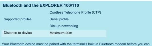
Your Bluetooth device must be paired with the terminal's built-in Bluetooth modern before you can make Bluetooth calls or transmit Bluetooth data. If you want to pair your device with the terminal, the default device name is "NERA-GW", and the default passkey is 0000 (four zeroes)..
