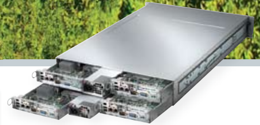
2U Twin 2 ™ 4 DP Nodes in 2U 375 GFLOPS/kW
