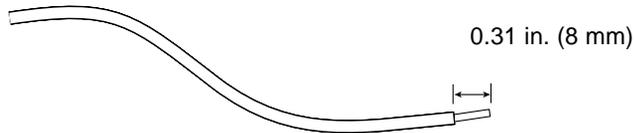
**FIGURE 3-2** Stripping the Insulation From the Wire
