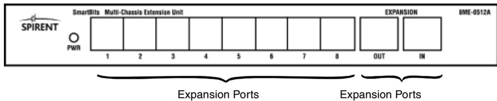
Figure A-6. Multi-chassis Extension Unit – Front View
