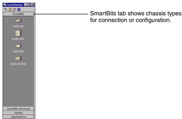
Figure 2-4. *SmartBits Tab (SmartWindow Launcher)*
