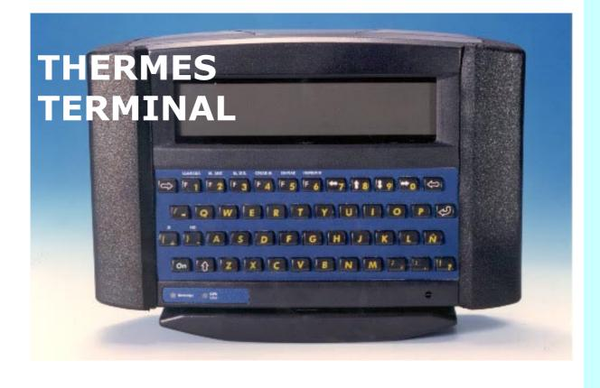
The **THERMES** GPS location terminal is a modular equipment for the location of mobile platforms using the constellation of GPS satellites. It may be adapted to any keyboard configuration, with the purpose of sending and receiving messages and information to and from the mobile units.
