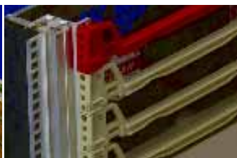
Keyable plastic guide rail.
