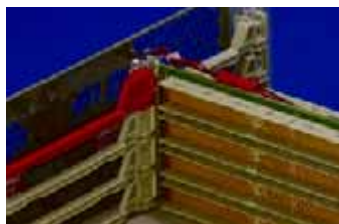
2 slots per U for CPCI/ VME boards at the front and rear.
