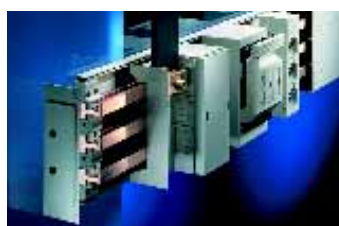
PLS end cover PLS busbar supports up to 1600 A, 3-pole PLS base tray sections
