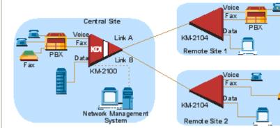
x is suitable for integrating all traffic requirements between two sites over a For connectivity between three or more sites, Kilomux supports Drop & In ariety of links. A dual link option supports both load sharing between the two and bypass used in "V", Ring or Chain topologies. s well as automatic backup with priority bumping.
