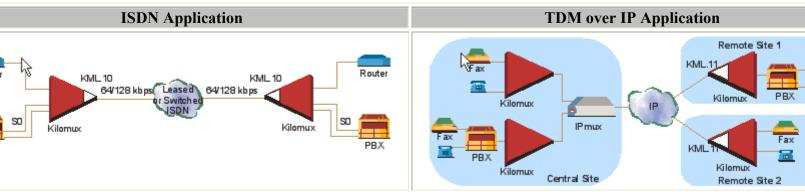
x enables connectivity over switched or leased line ISDN networks, tivity to ISDN switches, as well as extension of ISDN services to EDN premises.
