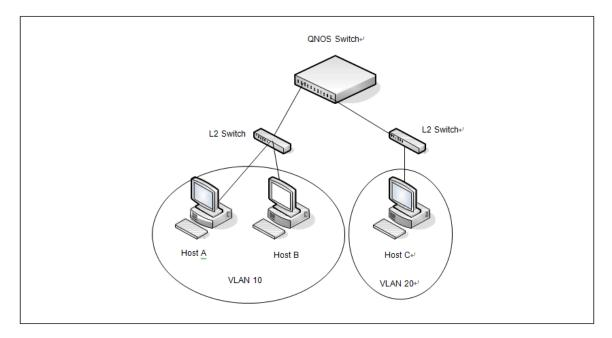
Figure 7-1: Inter-VLAN Routing
