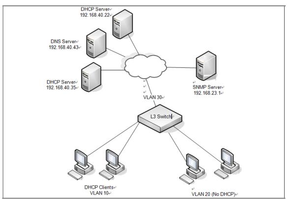
Figure 7-7: L3 Relay Network Diagram
