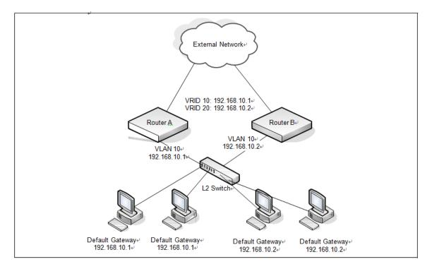
Figure 7-5: VRRP with Load Sharing Network Diagram
