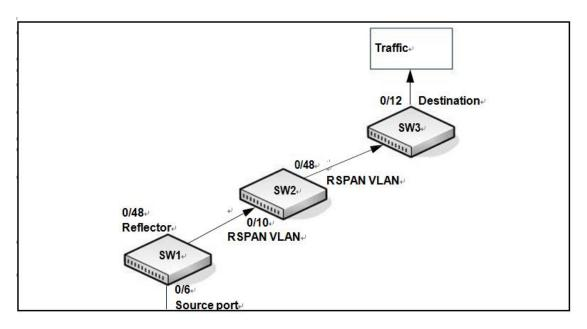
Figure 3-10: RSPAN Configuration Example
