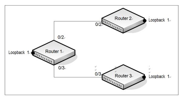
Figure 7-3: IP Unnumbered Configuration Example
