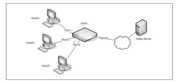
Figure 3-16: Switch with IGMP Snooping
