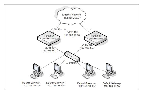
Figure 7-6: VRRP with Tracking Network Diagram
