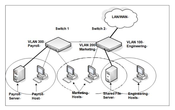
Figure 3-3: Network Topology for VLAN Configuration
