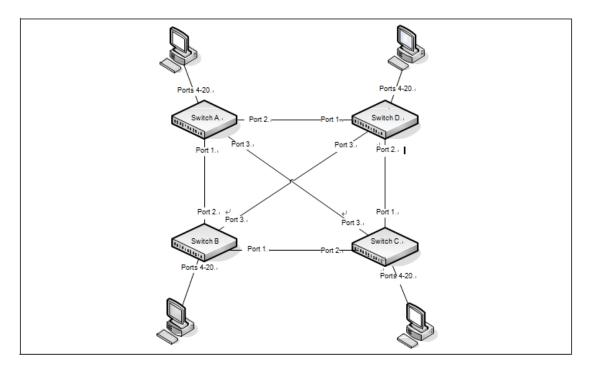
Figure 3-14: STP Example Network Diagram
