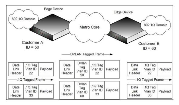
Figure 3-2: Double VLAN Tagging Network Example
