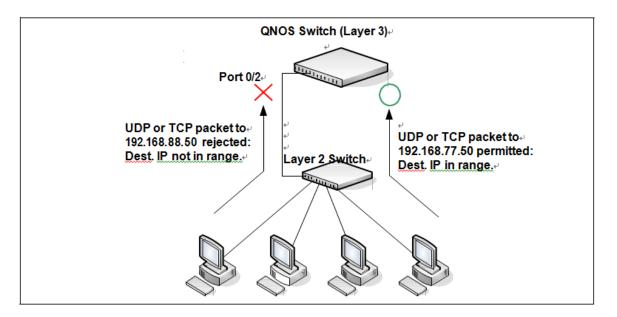
Figure 4-4: IP ACL Example Network Diagram
