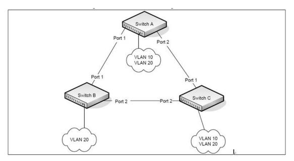
Figure 3-11: STP in a Small Bridged Network
