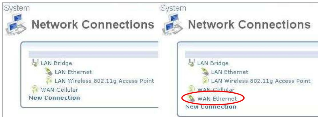
**Figure 5: Comparison between Old and New Network Connections page.**
