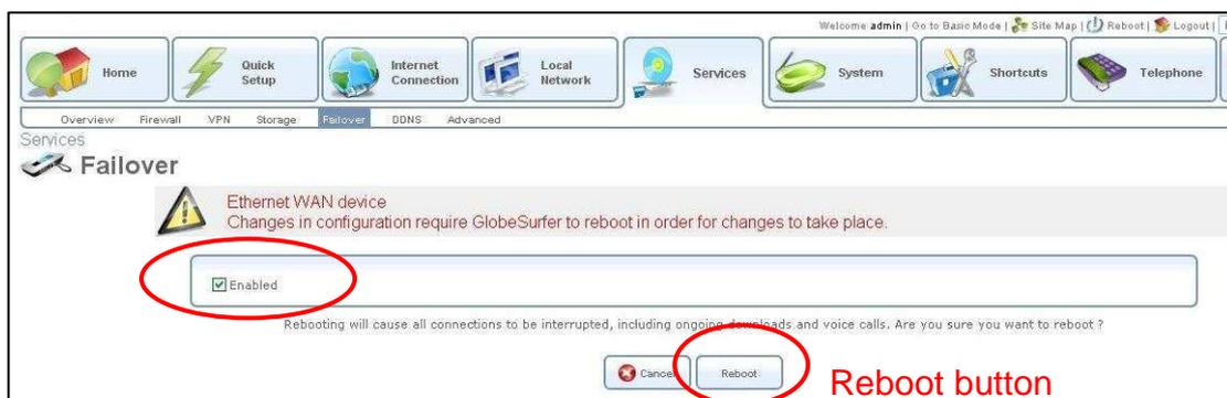
**Figure 3: Enabling Failover functionality.**
