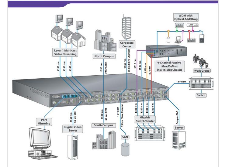
Establishing a data connection with a SFP Media Cross-Connect chassis is straightforward. Simply insert the SFP transceivers into the chassis and then via software management set the port-to-port connections, including port-to-multiport. For the NC316-XP32-3R, the interface data rate is also set.
