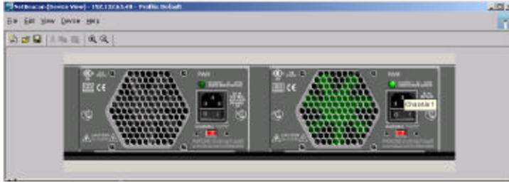
Power supply A has been disconnected. The fan has stopped running no longer shows as green.
