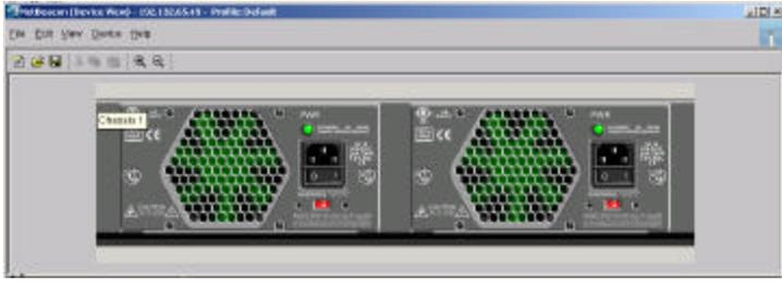
Double-clicking the chassis image in the upper half of the NetBeacon screen will show the rear of the chassis. Both power supplies are connected. Fans are operating normally and show as green in this view.
