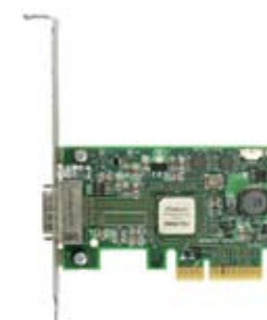
MHES14-XTC – 10Gb/s InfiniBand w/ PCI Express x4
