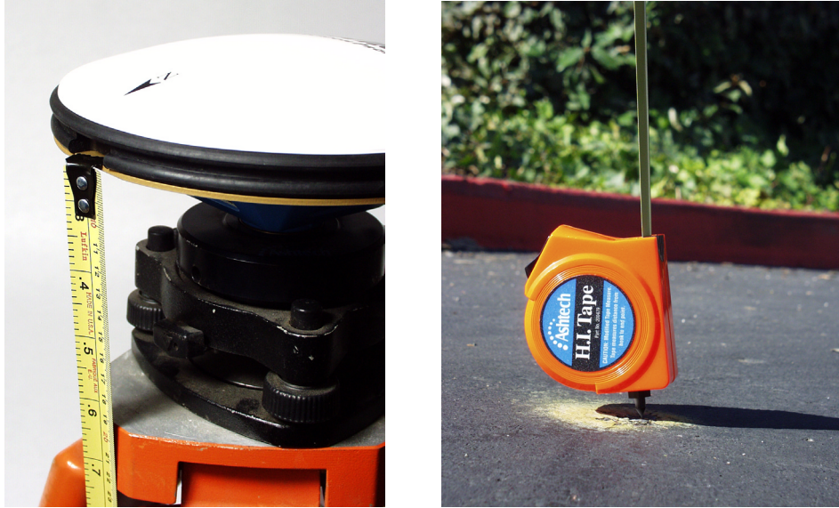
Figure 4.4 Measuring HI (Height of Instrument) of GPS Antenna
