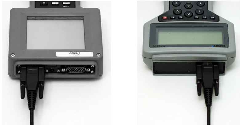
Figure 3.25 Handheld Computer with all Cables Connected
