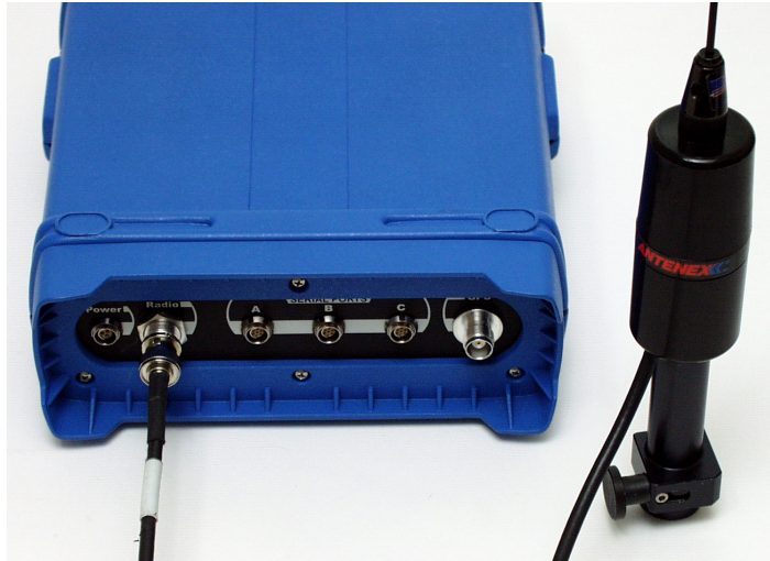
Figure 3.17 Rover Antenna Connected to Internal Radio
