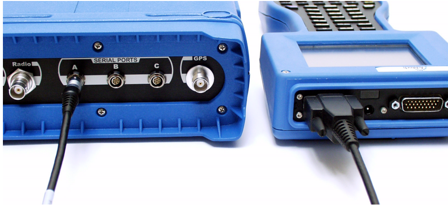
Figure 3.8 Communication Cable Connecting Z-Xtreme and Ranger Handheld
