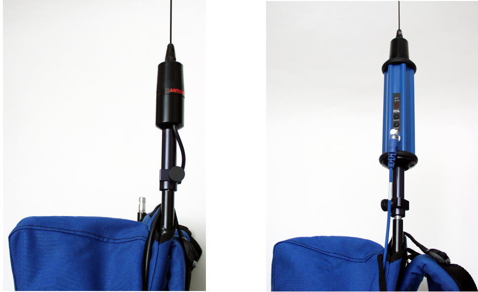
Figure 4.9 Rover Radio Antenna and Pacific Crest PDL Radios on Backpack
