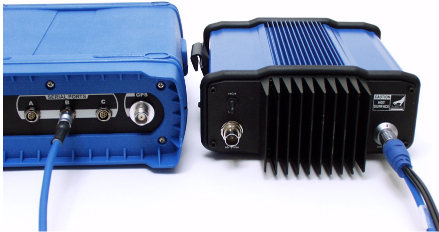
Figure 3.6 Communication Cable Connecting Z-Xtreme Receiver and Pacific Crest Radio
