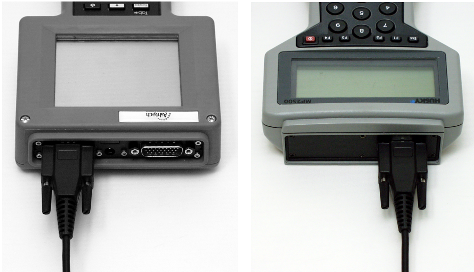
Figure 3.15 Handheld Computer with all Cables Connected
