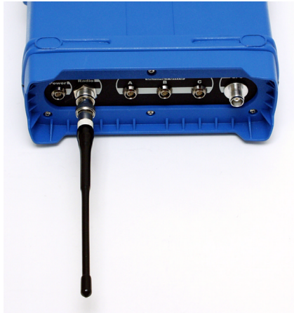
Figure 4.11 Rubber Duck Antenna Mounted to Z-Xtreme
