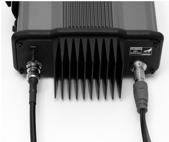
Figure 3.14 Pacific Crest Radio with all Cable Connections
