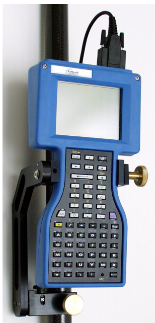
Figure 4.12 TDS Ranger Handheld Mounted on Rover Pole
