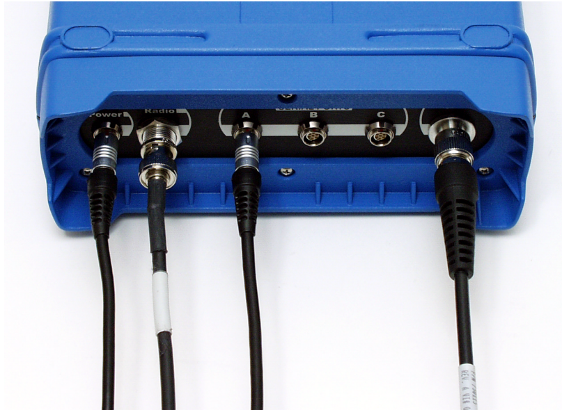
Figure 3.23 Cable Connections for Z-Xtreme Rover with Internal Radio
