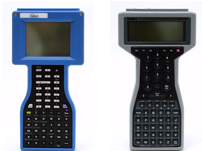
Figure 2.8 Handheld Computers: TDS (left), Husky MP2500 (right)
