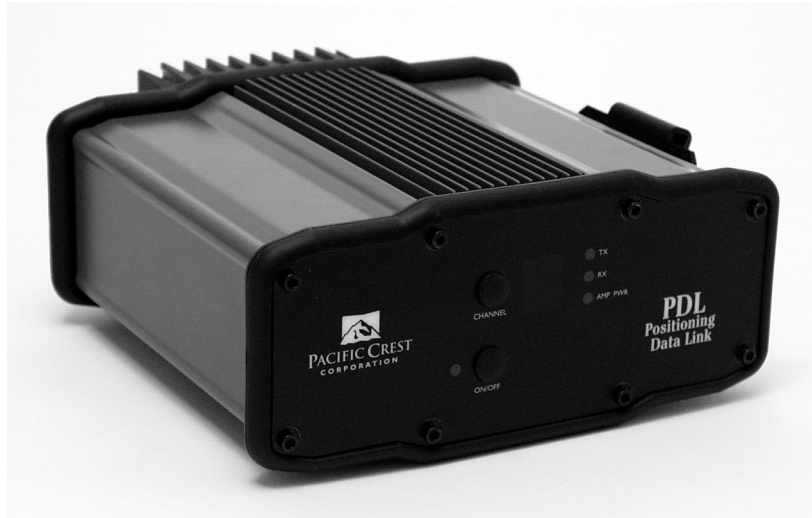
Figure 2.4 Pacific Crest UHF/VHF Base Radio
