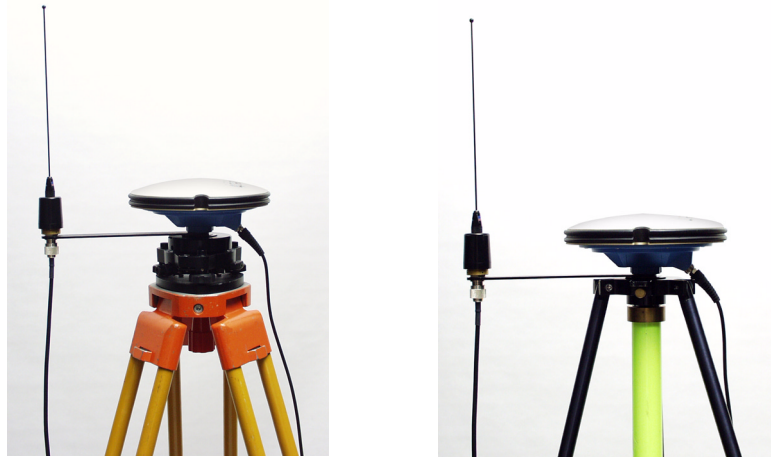
Figure 4.3. Base Antennae Mounted on Conventional (left) and GPS Tripods (right)
