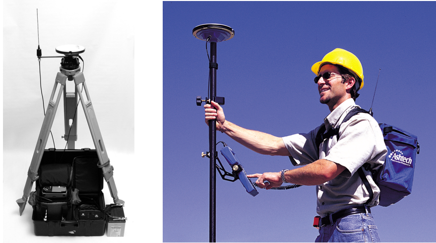
Figure 1.1 RTK Setup for GPS Surveying
