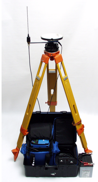
Figure 4.6 Base System Ready to Survey
