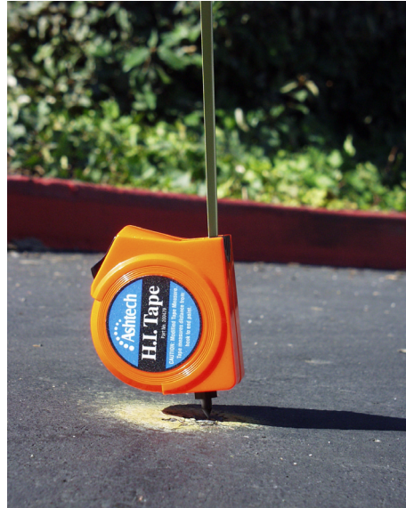
Figure 4.5 Measuring HI (Height of Instrument) of Base GPS Antenna
