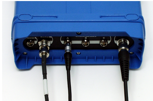
Figure 3.29 Fully Connected Pole-mounted Rover GPS Receiver
