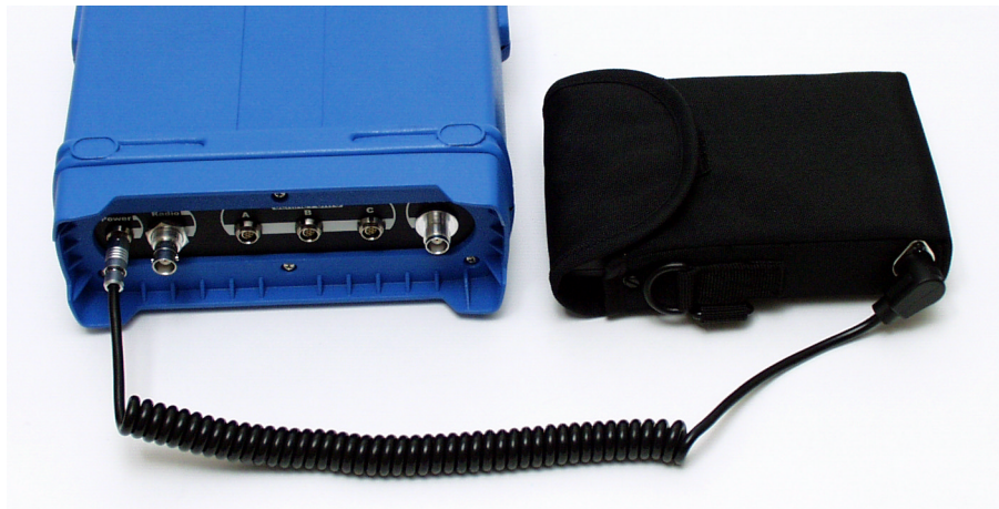
Figure 3.10 Power Cable Connecting Z-Xtreme and External Battery
