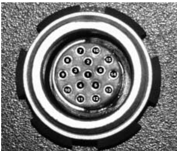
Figure 2.4. Serial Port Pin Layout
