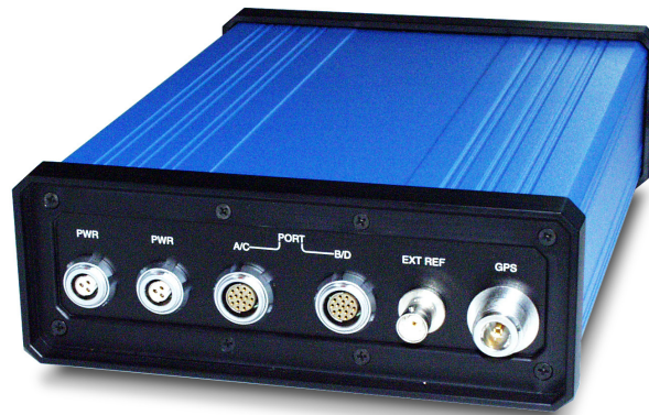
Figure 2. \mu Z-CGRS Rear Panel
