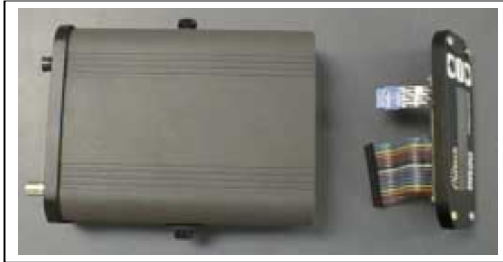
Figure 2 – BR2G Receiver with Front Panel Removed
