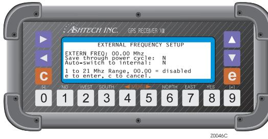
**Figure 4.12:** External Frequency Setup Screen
