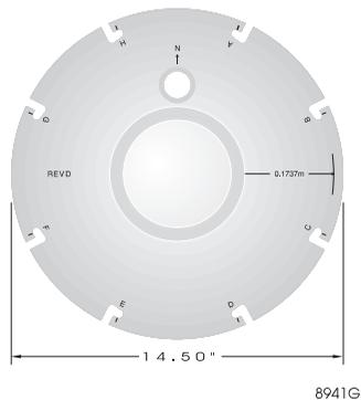
**Figure 2.4:** Antenna Dimensions
