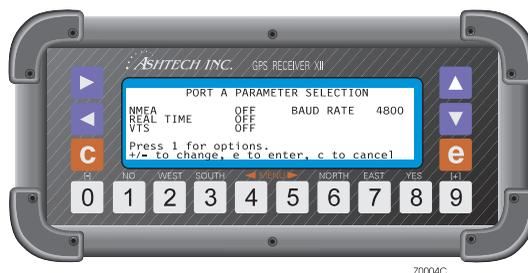
**Figure 5.2:** Port A Parameter Selection Screen
