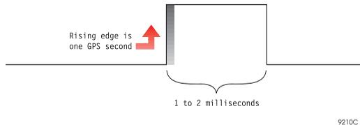
**Figure 4.14:** Rising Edge Pulse Alignment
