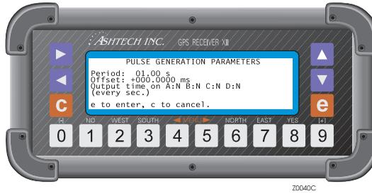
**Figure 4.13:** Pulse Generation Parameters Screen
