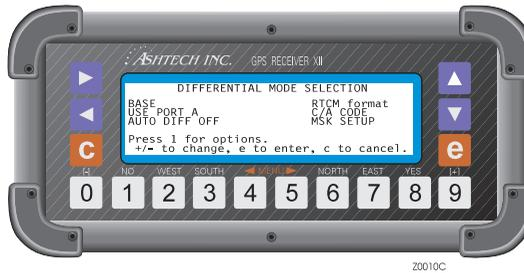
Figure 3.9: Differential Mode Selection Screen
