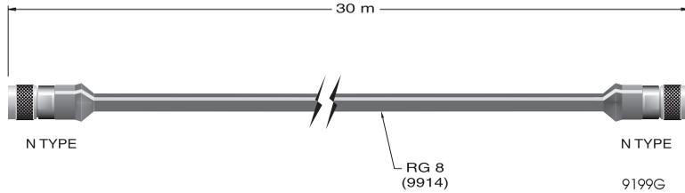
**Figure 9.1:** Antenna Cable
