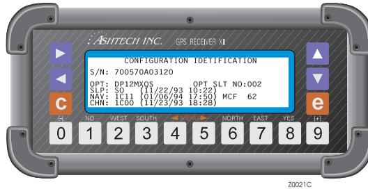
**Figure 4.39:** Configuration Identification Screen
