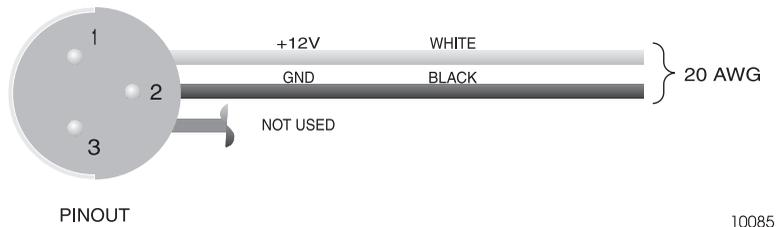
**Figure 9.3:** Power Cable Pinouts
