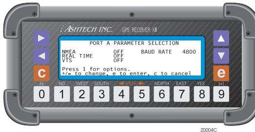
Figure 4.11: Port A Parameter Selection Sub-screen
