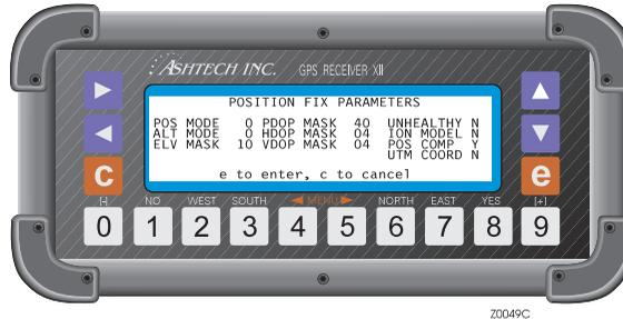
**Figure 4.7:** Position Fix Parameters Screen
