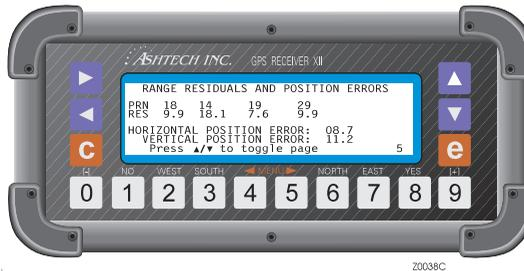
**Figure 4.21:** Range Residuals and Position Errors Screen
