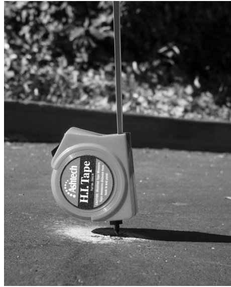
Figure 4.4. Measuring HI (Height of Instrument) of GPS Antenna
