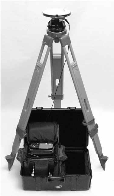
Figure 4.5. Z-Xtreme Survey System Performing a Static Survey
