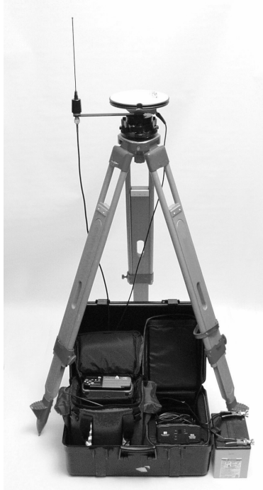
Figure 4.6. Base System Ready to Survey
