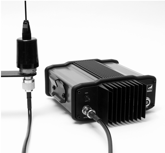
Figure 3.4. Cable Connected to Pacific Crest Radio and Base Radio Antenna
