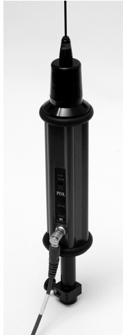
Figure 3.24. Pacific Crest Rover Radio with all Cable Connections
