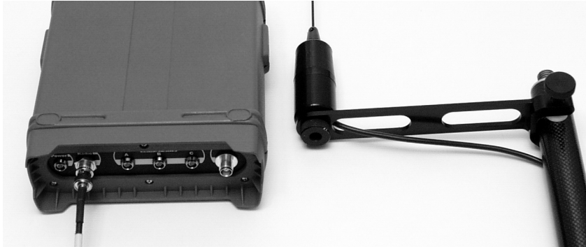
Figure 4.10. Radio Antenna Mounted On Pole and on Back of Receiver
