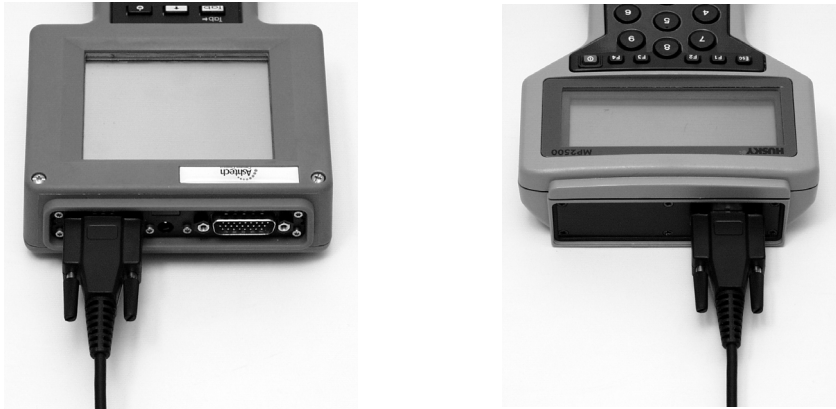
Figure 3.30. Fully Connected Handheld Computer
