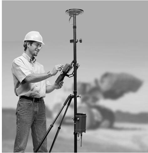
Figure 4.15. Pole-mounted Rover System Ready to Survey
