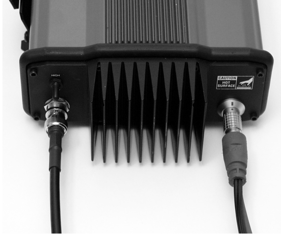
Figure 3.14. Pacific Crest Radio with all Cable Connections
