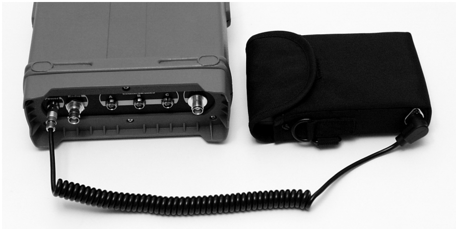
Figure 3.10. Power Cable Connecting Z-Xtreme and External Battery
