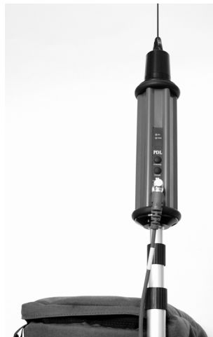
Figure 3.18. Pacific Crest PDL Rover Radio with Antenna
