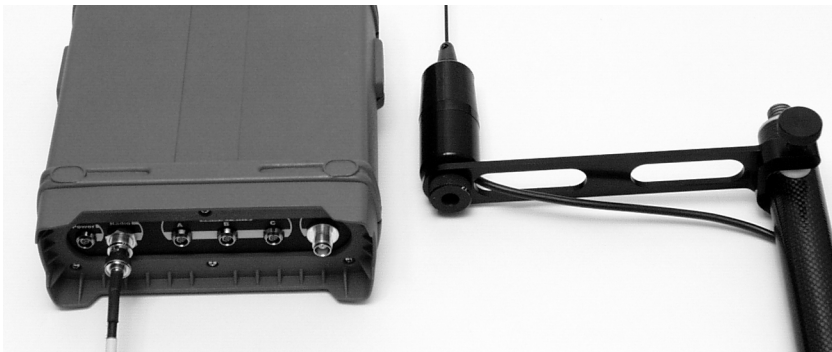
Figure 3.27. Rover Radio Antenna Cable Connected to Internal Radio and Radio Antenna
