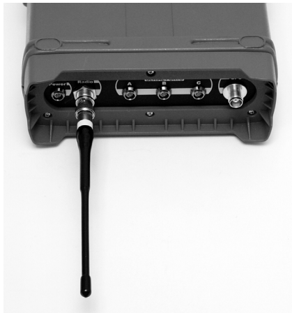
Figure 4.11. Rubber Duck Antenna Mounted to Z-Xtreme
