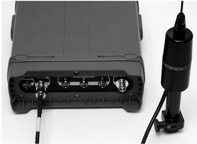
Figure 3.17. Rover Antenna Connected to Internal Radio
