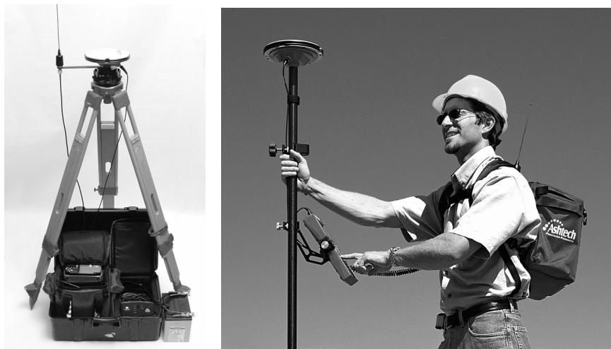
Figure 1.1. RTK Setup for GPS Surveying
