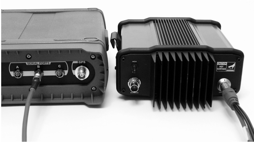
Figure 3.6. Communication Cable Connecting Z-Xtreme Receiver and Pacific Crest Radio
