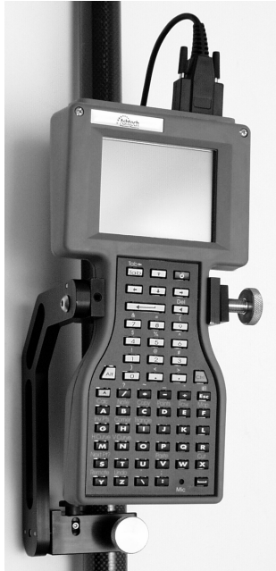
Figure 4.12. TDS Ranger Handheld Mounted on Rover Pole
