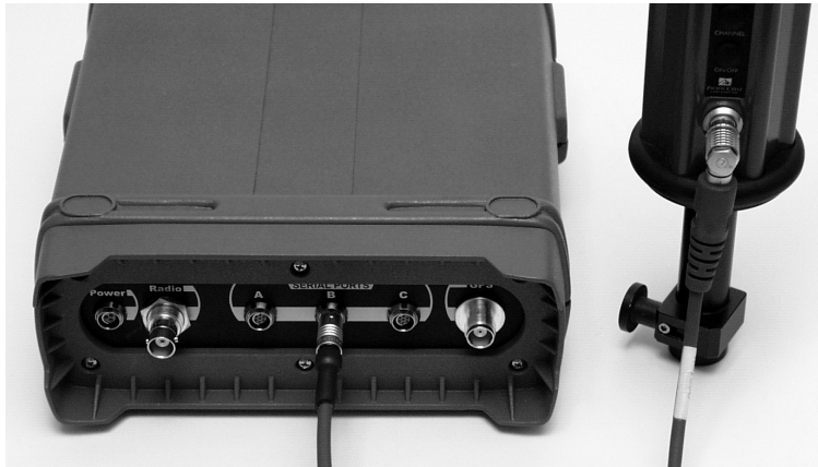
Figure 3.20. Communication Cable Connecting Z-Xtreme and PDL Rover Radio
