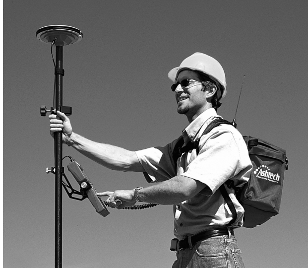
Figure 4.14. Backpack Rover System Ready to Survey
