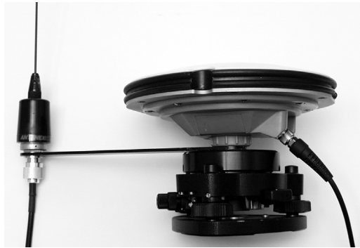
Figure 4.4. Mounted Base Radio Antenna
