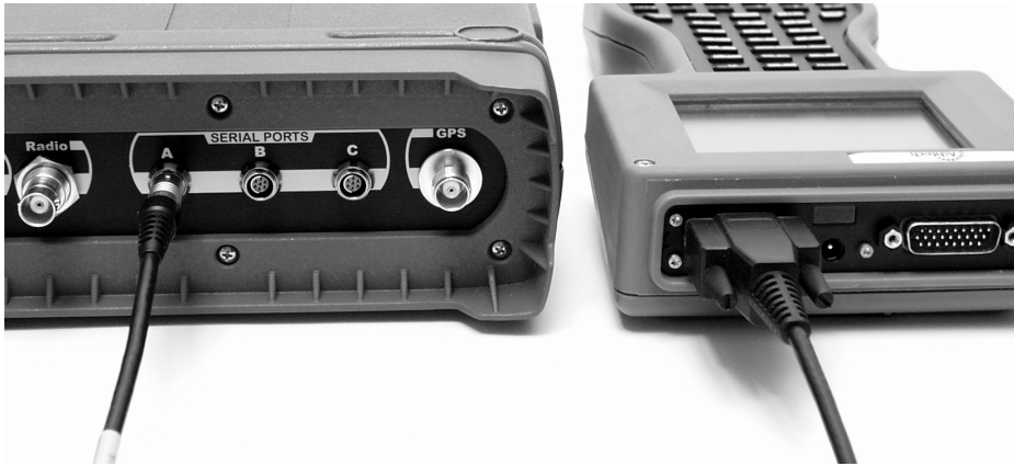
Figure 3.8. Communication Cable Connecting Z-Xtreme and Ranger Handheld
