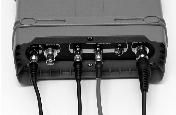
Figure 3.22. Cable Connections for Z-Xtreme Rover with External Radio
