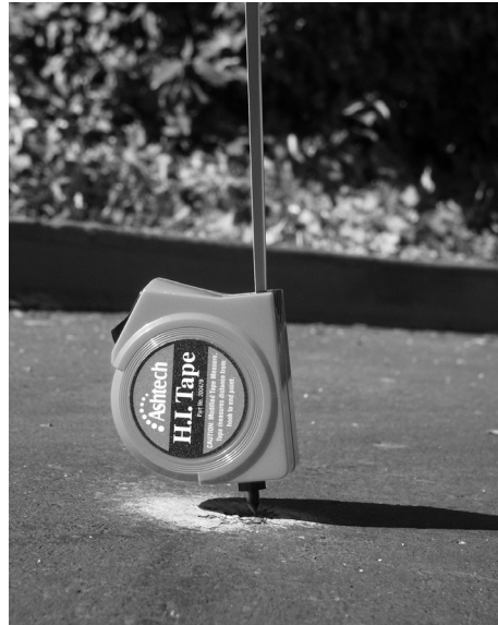
Figure 4.5. Measuring HI (Height of Instrument) of Base GPS Antenna
