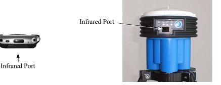
Figure 2.23 Handheld and Locus Infrared Ports
