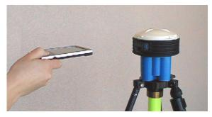
Figure 2.24 Communication between Handheld and Locus IR Ports
