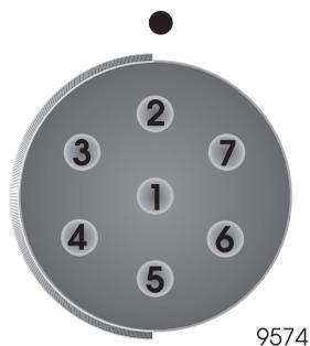
**Figure 1.4:** SERIAL Data Connector Pin Configuration
