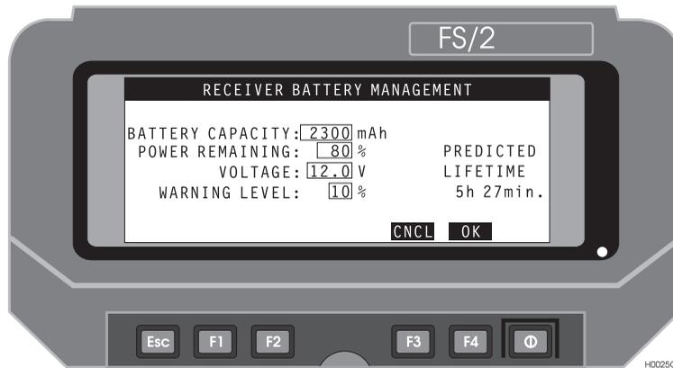
**Figure 4.4:** Receiver Battery Management Screen (BATT)
