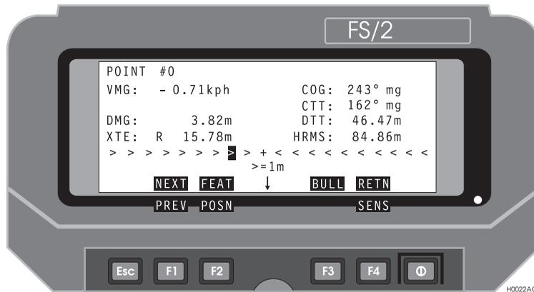
**Figure 4.52:** Horizontal Navigation Screen (NAVI)
