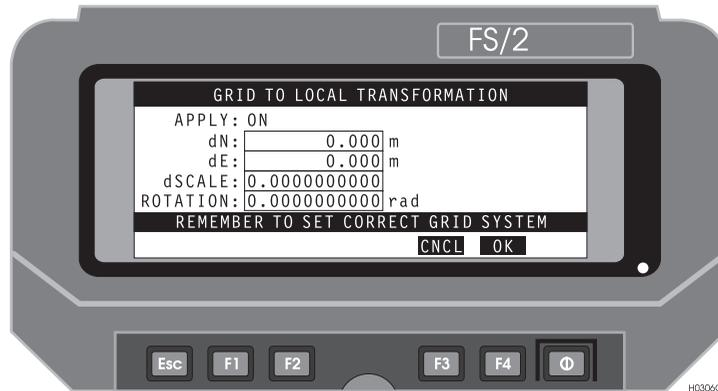
**Figure 4.47:** Grid to Local Transformation Screen (LOCL)
