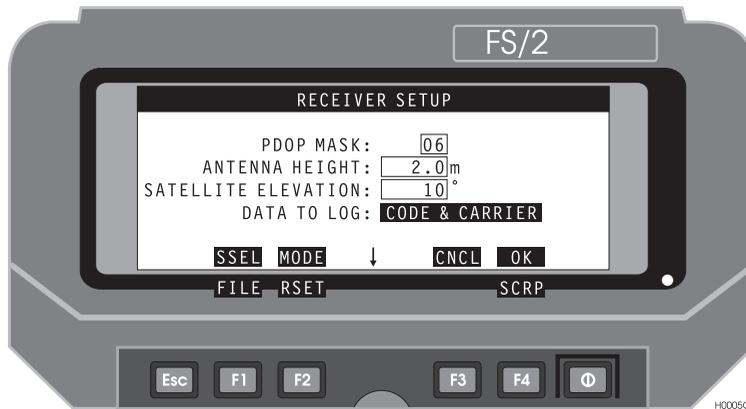
**Figure B.2:** Receiver Setup Screen
