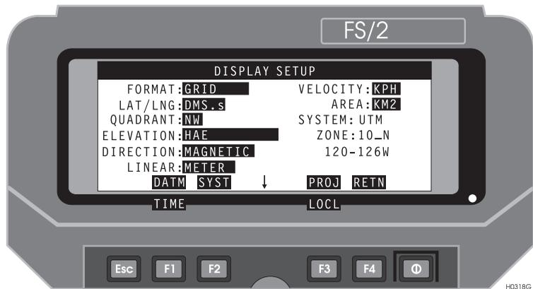
**Figure 3.44:** Display Setup Screen.
