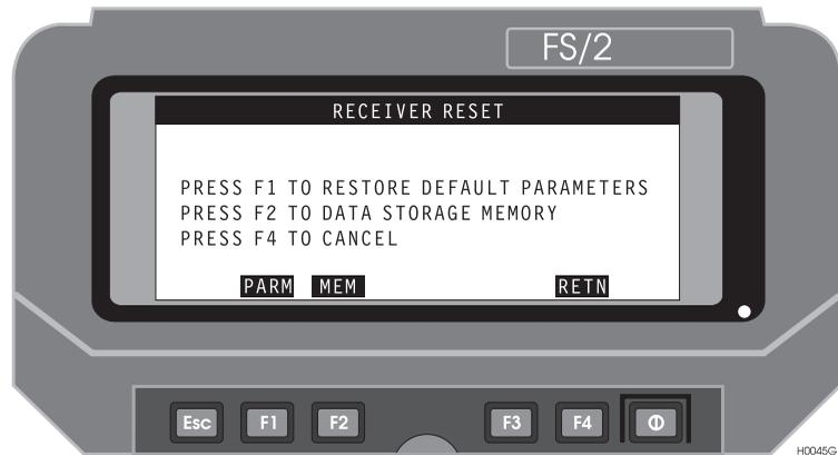
**Figure 4.32:** Receiver Reset Screen (RSET)
