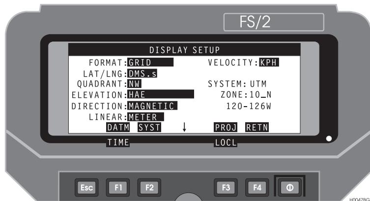
**Figure 4.35:** Display Setup Screen (DSST) Grid Format
