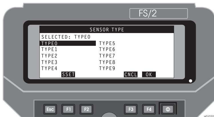
**Figure 4.20:** Sensor Type Screen (TYPE)
