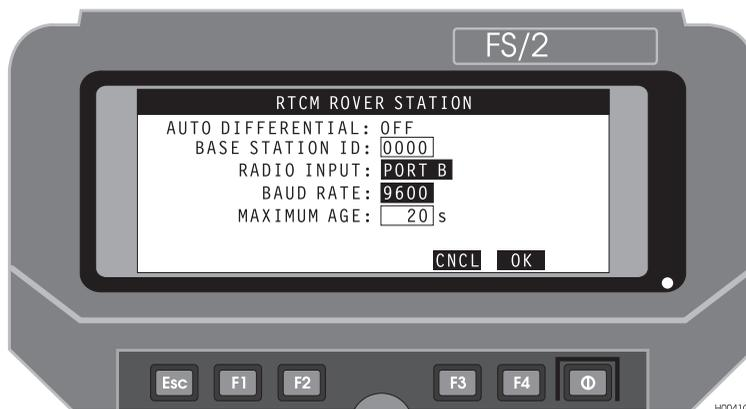
**Figure 4.28:** RTCM Rover Station Screen (ROVR)
