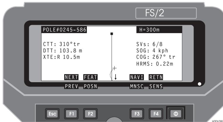
**Figure 4.54:** Vertical Navigation Screen (LINE)
