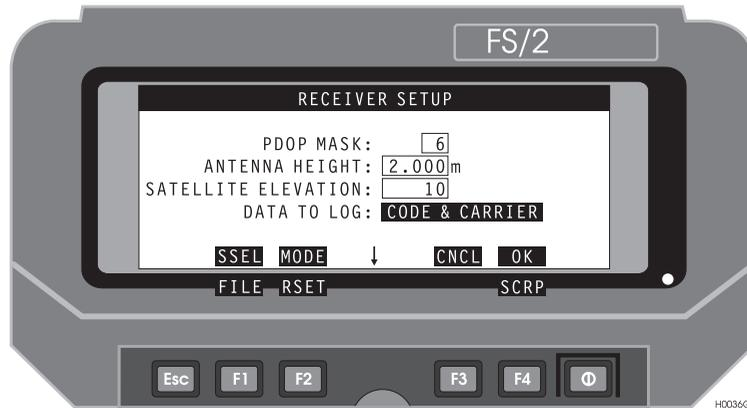
**Figure 4.23:** Receiver Setup Screen (RCVR)
