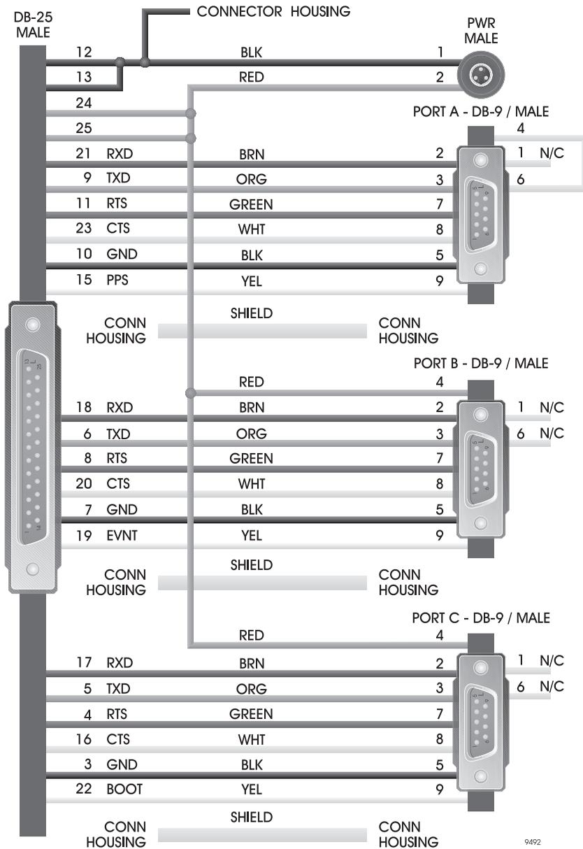
Figure D.2: Interface Cable Pinout Diagram
