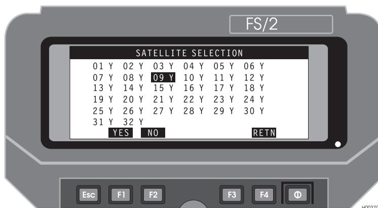
**Figure 4.24:** Satellite Selection Screen (SSEL)
