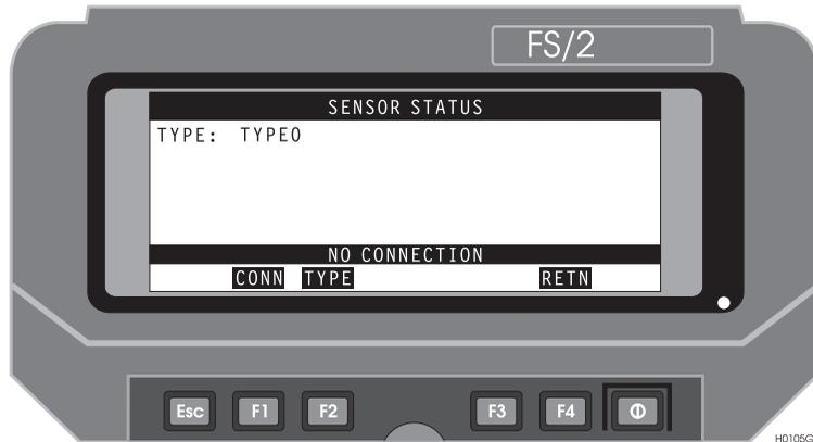
**Figure 4.18:** Sensor Status Screen (SENS) With No Connection
