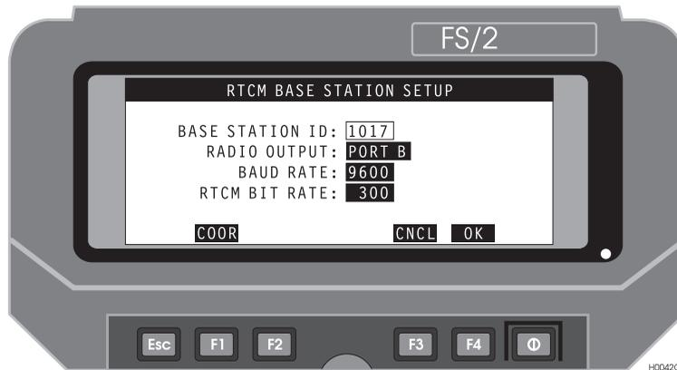
**Figure 4.29:** RTCM Base Station Screen (BASE)
