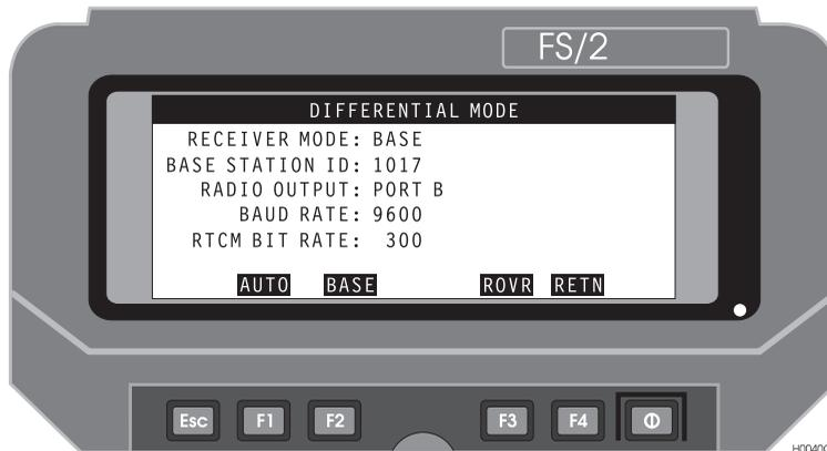
**Figure 4.27:** Differential Mode Screen (MODE) - Base
