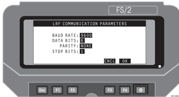
**Figure 4.17:** LRF Communication Parameters Screen
