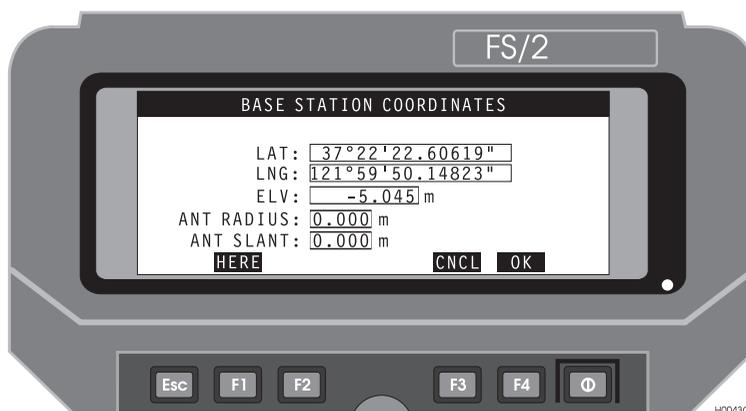
**Figure 4.30:** Base Station Coordinates Screen (COOR)
