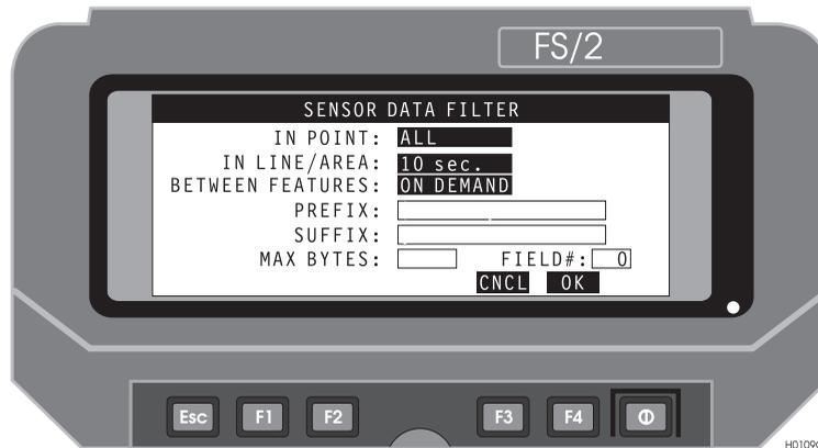
**Figure 4.22:** Sensor Data Filter Screen (FLTR)
