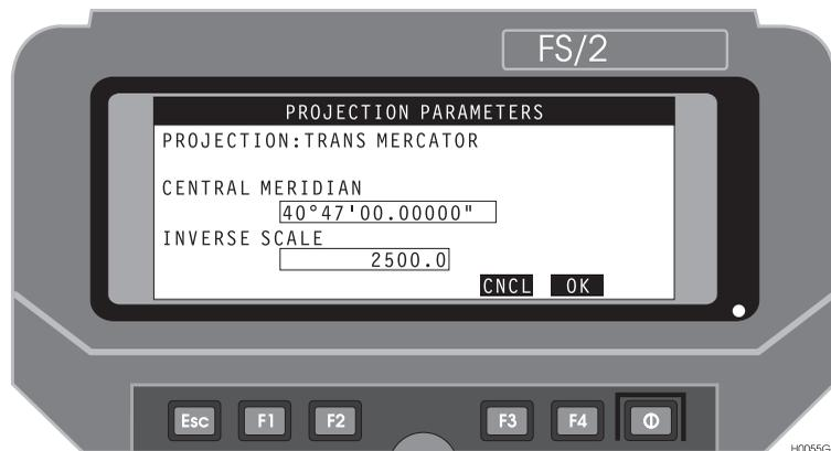
**Figure 4.43:** Projection Parameters (PARM) - Trans Mercator
