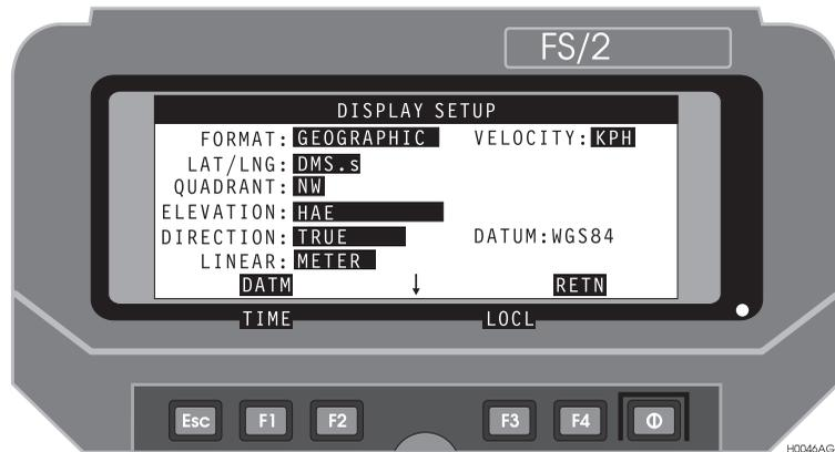
**Figure 4.34:** Display Setup Screen (DSST) Geographic Format
