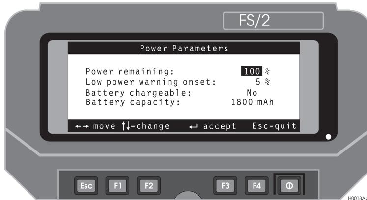
**Figure C.4:** Power Parameters - Screen 2
