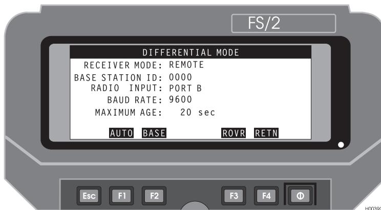
**Figure 4.26:** Differential Mode Screen (MODE) - Remote
