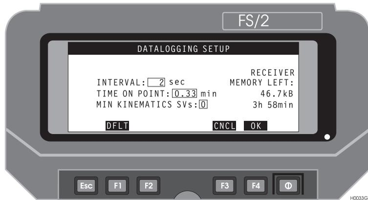
**Figure 4.11:** Datalogging Setup Screen (LGST)
