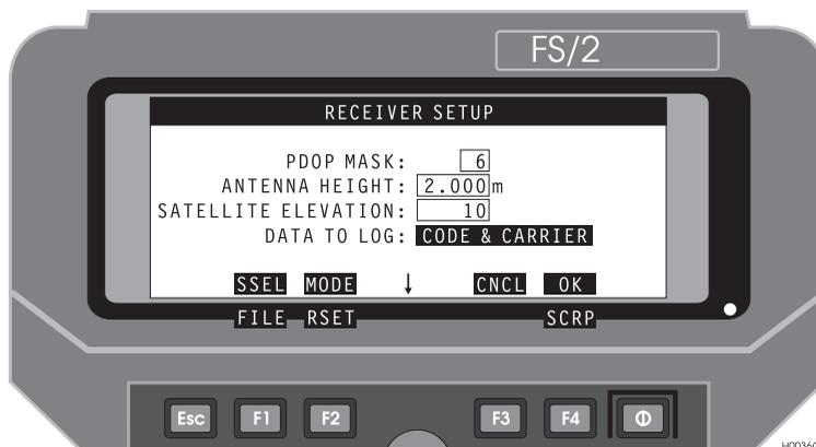
**Figure 3.11:** Receiver Setup Screen
