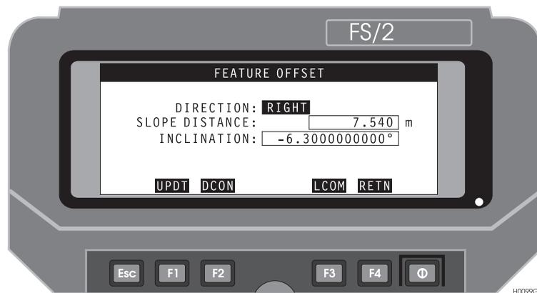
**Figure 4.16:** Feature Offset Screen - Line of Travel
