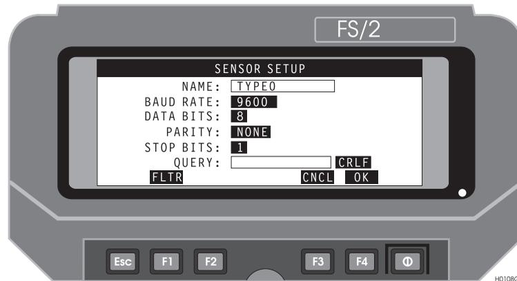
**Figure 4.21:** Sensor Setup Screen (SSET)
