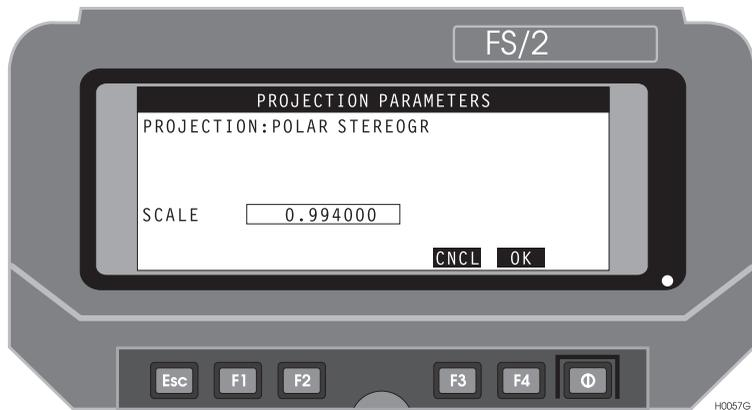
**Figure 4.45:** Projection Parameters (PARM) - Polar Parameter
