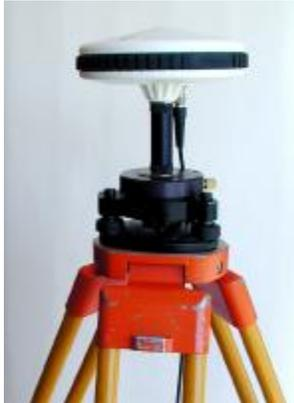
**Figure 3.10** GPS Antenna Mounted on Tripod using Tribrach and Extender
