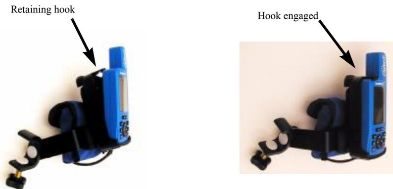
**Figure 3.11** Mounting ProMark2 into Field Bracket Cradle
