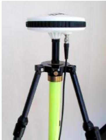
**Figure 1.15** Fixed-Height GPS Tripod with Extender and GPS Antenna
