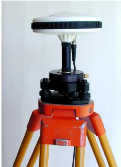
**Figure 1.12** Tripod, Tribrach, and Tribrach Adapter
