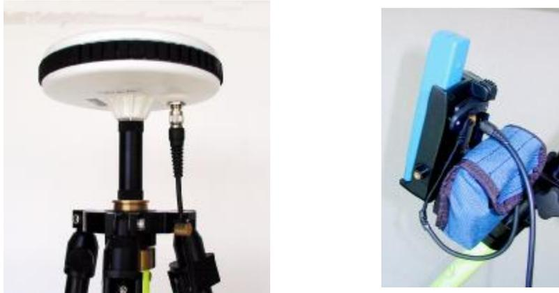
**Figure 3.13** Antenna Cable Connection at the Antenna and Receiver
