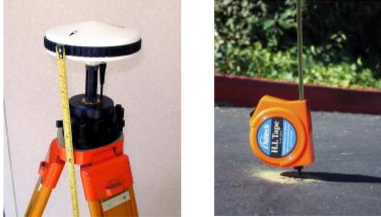
**Figure 3.14** Measuring HI (Height of Instrument)
