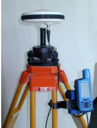
**Figure 3.12** Field Bracket on Tripod
