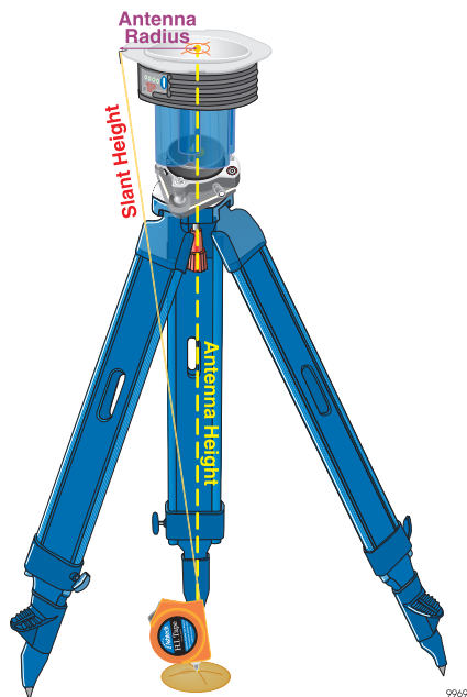
Figure 3.34: Measuring Slant and Offset
