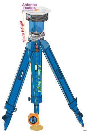
Figure 3.2: Tape Measure In Use
