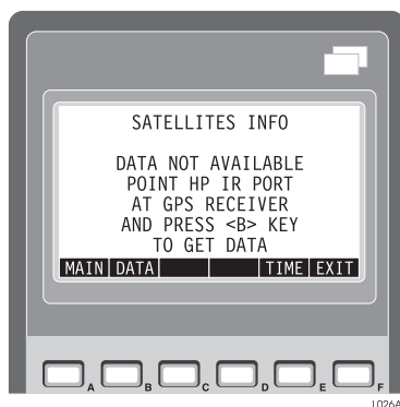
Figure 3.28: Satellites Info Screen Before Reading Information
