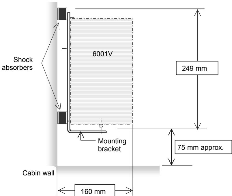
When choosing a place inside the cabin, remember the distance to the UHF antenna should remain as short as possible (a 6-m coaxial cable is provided for the connection of this antenna to the 6001V).
