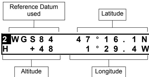
If no solution is available ("HOLD" displayed on screen No.0), this screen will display the "initial position", as defined by the configuration, or the latest position computed in case of lasting solution unavailability, due to reception loss for example.
