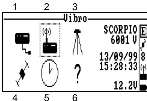
Use the vertical- or horizontal-arrow keys ( $\uparrow$ ,  $\downarrow$ ,  $\rightarrow$ ,  $\leftarrow$ ) to select an icon. The selected icon is surrounded by dotted lines. Then press  $\downarrow$  to enter the corresponding function. Alternately, you can directly enter a function by pressing the corresponding numeral key (see figures 1 to 6 in the screen example above)
