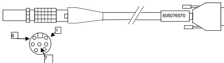
A is a 7-contact JKX FD 1G 07 MSSDSM (5011253) plug with JBX1 MPN (5080359) sleeve. Manufacturer: FCI.
