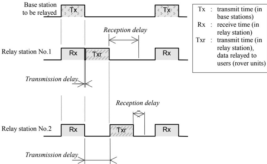
*Reception delays* are adjusted so as to avoid data links between relays if they are mutually within range.
