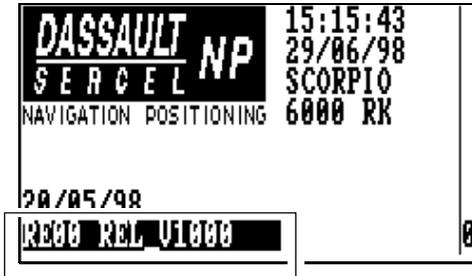
After pressing ↵, use the ↑ or ↓ key to list the versions of the different parts installed.
