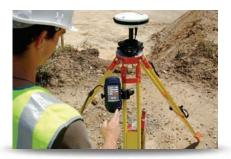
As with the original ProMark3 receiver, post-processing features are included in ProMark3 RTK. Raw data, simultaneously recorded during RTK jobs, can also be post-processed via the GNSS solutions office software for superior survey integrity.
