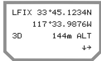
Earlier position fixes are numbered in reverse order (the more recent the fix is, the higher the number is). Continue pressing the **RIGHT ARROW** to scroll through the earlier fixes and back to LFIX. At any time, press the **DOWN ARROW** to view the second and third position screens showing PDOP and SQ's.
