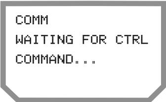
This message is displayed briefly during data upload. It indicates that the unit is receiving the selected file. Once upload is complete, the "WAITING FOR CTRL COMMAND" message is displayed. Press the **RIGHT ARROW** twice to return to the initial AUX 5 display.
