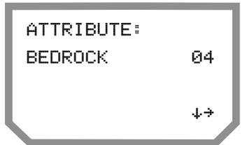
In order to make the key assignments in a particular attribute file active, you must use the **DOWN ARROW** from the attribute file screen to make the file the ACTIVE FILE. Note that only one attribute file may be made active at any time, (i.e., activating a file will deactivate any other active files).
