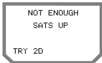
**Unit Searches Constantly.** If the unit has an almanac and is unable to locate satellites, it searches continually until a satellite is found.
