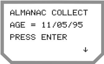
Age is the date that is assigned to almanac information that is broadcast from a specific satellite on a specific day by GPS operators. Generally, age is within six days of the actual date of collection. If the unit has no almanac, the second line is blank.
