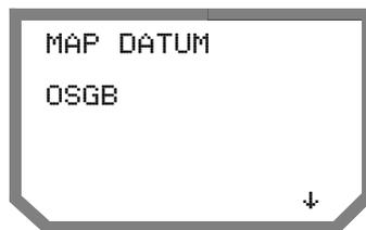
The unit stores the positions it calculates (and the waypoints you enter) in the WGS84 datum and as height above ellipsoid (HAE). A position is converted from WGS84 and HAE to the systems you have selected when it is displayed. Since Lat/Lon and UTM are global systems, they can be used to describe locations anywhere on earth. A position in the area described by British grid can therefore be described in Lat/Lon, UTM, or British grid. It cannot be described in UPS or Irish grid.
