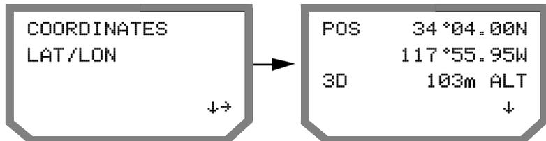
You may also select how Lat/Lon coordinates are displayed. You may select degrees/minutes and display minutes to two or four places, or select degrees/minutes/seconds and display the two-digit seconds with or without two decimal places. The following table shows the same position in each format.
