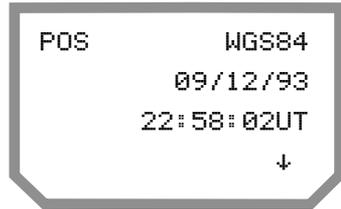
Press the **DOWN ARROW** again to see which satellites were used to compute the position, the SQ, and the PDOP of the fix. (See Appendix 8 and 9 for a description of PDOP and SQ.)
