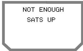
If you are operating with the Battery Saver on, the unit shuts itself off if it cannot locate enough satellites for a fix.
