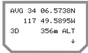
Note that the display uses the same format as a waypoint. If the number of fixes selected has not yet been reached and ENTER is pressed from the "WAIT" display, a confirmation message appears stating to press ENTER to stop the session or CLEAR to continue.
