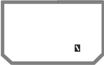
**Accuracy warning:** The Position Dilution of Precision (PDOP) of the position fix is 10.1 or more; the fix is not accurate, and should not be used to navigate by. This symbol appears on all screens of the affected position fix.
