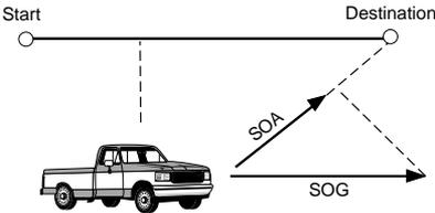
A vector component of ground speed (SOG) towards the destination. Abbreviated as SOA. Displayed when NAV is pressed and after three position fixes have been taken.
