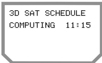
When the computations are complete, the unit displays the "window of availability." This is when there will be enough satellites to obtain a position fix.
