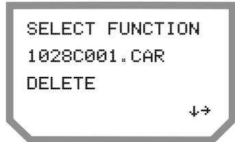
To erase all or selected portions of the unit's memory, press the **DOWN ARROW**. If you press CLEAR now, all of the unit's memory is erased. Press the **RIGHT ARROW** to scroll through the selections listed below.
