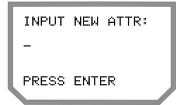
Type in the new attribute (up to 72 characters) with the alphanumeric keys. Press **ENTER** when entry is completed to return to the Attribute screen with the newly entered attribute displayed.
