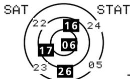
The concentric circles indicate elevation, or height above the horizon. The outer circle is the horizon, or 0° elevation. The next two circles are 30° and 60°, respectively. The center is 90°, or straight up.
