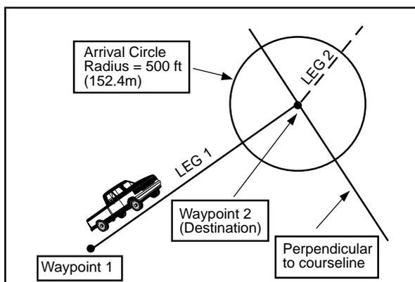
In the automatic route mode, the unit switches from the current leg to the next when you cross an imaginary line that runs through the destination waypoint and is perpendicular to the courseline. All navigation information is now referenced to the destination waypoint of the new leg.
