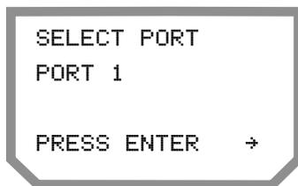
If you don't have the port set to output NMEA (Setup 7), you can override the port setting by just pressing ENTER when you access this function.
