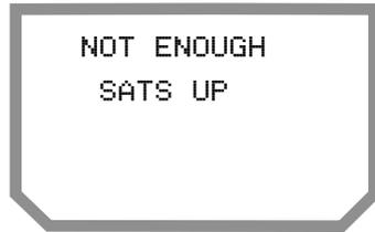
The unit devotes all ten channels to the search for the satellite the almanac indicates is directly overhead, given your last fix or initial position. This generally takes a few seconds. If the satellite cannot be located, the unit looks for the satellite with the next highest elevation. Searching for the highest satellite greatly shortens the length of time required to obtain a position fix.
