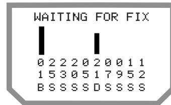
Throughout the search and acquisition of satellites the receiver status screen monitors the activity of all ten channels. (You may also access the receiver status screen at any time with AUX 1.). Refer to the following illustration to interpret this screen.
