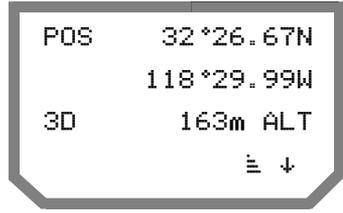
**Old Data.** The unit automatically updates its position every second. If a satellite signal is lost, or a satellite sets or becomes obstructed, the unit switches to other satellites to update the fix. If other satellites are not available, the unit cannot update the position fix.
