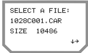
To rename a file, press the **ENTER**. Key in a new filename, followed by **ENTER**. The file is renamed, and the unit returns to the initial AUX 11 display.
