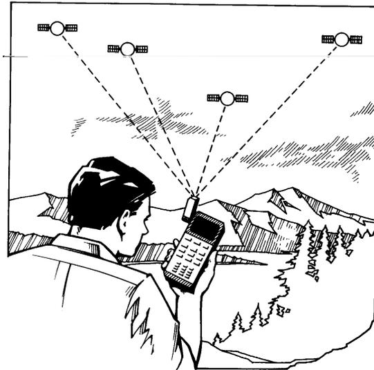
**Give the Antenna a Direct View of Satellites**
