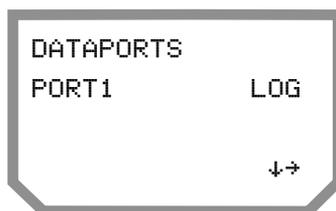
Next, use the **RIGHT ARROW** to select the baud rate for port 1. Select 9600, 19.2, 38.4, 115, 1200, 2400, or 4800. After you have set the ports, press the **RIGHT ARROW** to select DONE.
