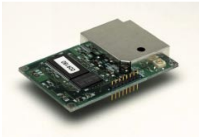
Figure 1.5: G8 Version 3, OEM Board with Stackable I/O Connector
