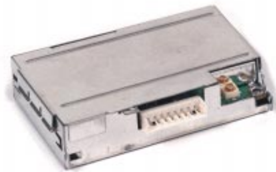
Figure 1.1: G8 Version 1, OEM Board with Mechanical Shield Case and Cable Ready I/O Connector
