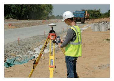
Stop & go surveys are simplified with ProMark3. The portability and the user-friendly interface enable a one-man crew to perform quick and reliable surveys.
