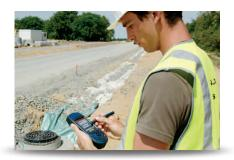
ProMark3 RTK enables you to take any supported GIS file into the field. Easily navigate to field infrastructure for reckon and mapping. Update your GIS data and transfer the file back to the office GIS for the customer.
