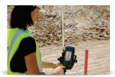
ProMark3 RTK can be used as a rover only, connected to a real-time network. A Bluetooth connection can be established between ProMark3 RTK and a cellular phone.
