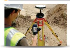
As with the original ProMark3 receiver, post-processing features are included in ProMark3 RTK. Raw data, simultaneously recorded during RTK jobs, can also be post-processed via the GNSS solutions office software for superior survey integrity.
