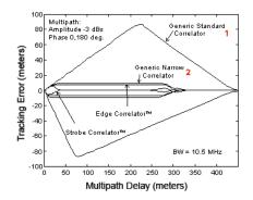
The horizontal axis of the plot show the multipath delay, this is the extra distance that the reflected signal travels compared to the direct signal. The vertical axis shows the induced range error caused by a multipath signal with the indicated delay.
