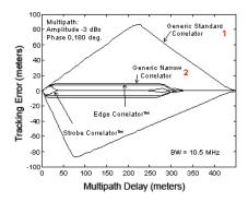
The horizontal axis of the plot show the multipath delay, this is the extra distance that the reflected signal travels compared to the direct signal. The vertical axis shows the induced range error caused by a multipath signal with the indicated delay.
