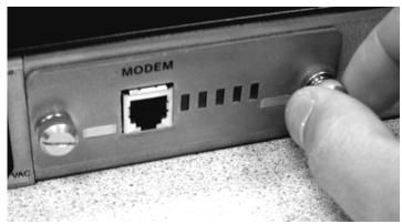
Figure 6-1. Installing a Modem Card in the SCSxx20
