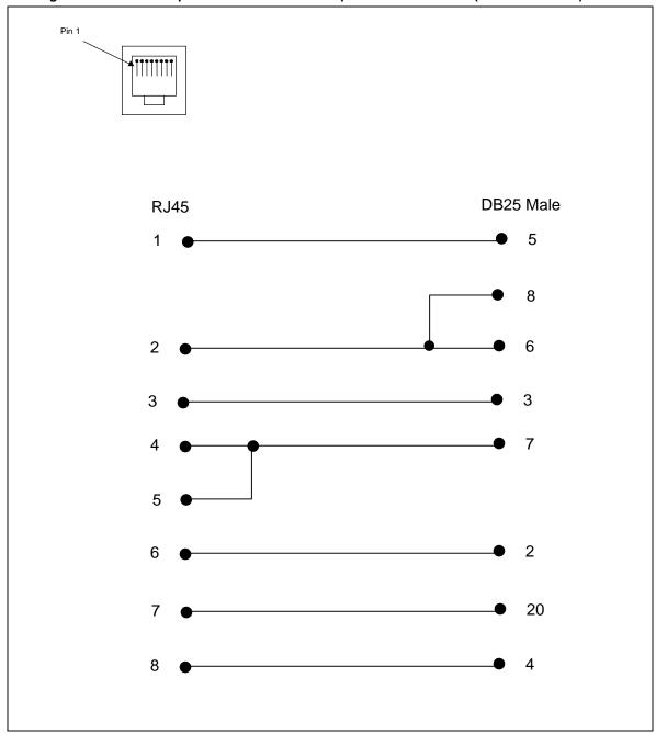
Use PN 200.2066A adapter with a dumb terminal or with most SUN applications.
