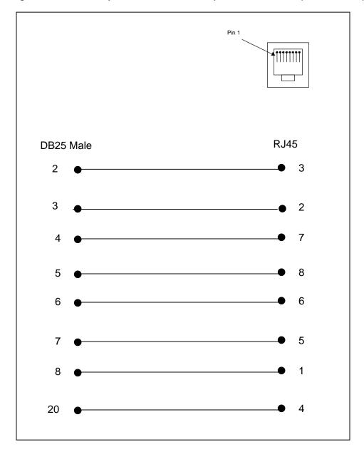
Use PN 200.0066 adapter with a dumb terminal or with most SUN applications.
