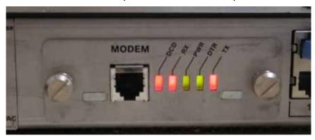
A red LED indicates the "inactive" state, and a green LED indicates the "active" state. The **PWR** LED should always be green when the system is on.
