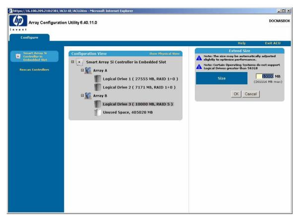
Figure 1 Expanding a LUN (Smart Array only)
