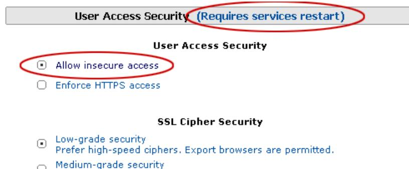
*Figure 1.4* Allowing insecure access so the BIG-IP can offload the SSL traffic
