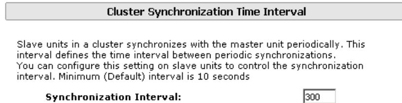
**Figure 1.3** Configuring the synchronization time interval
