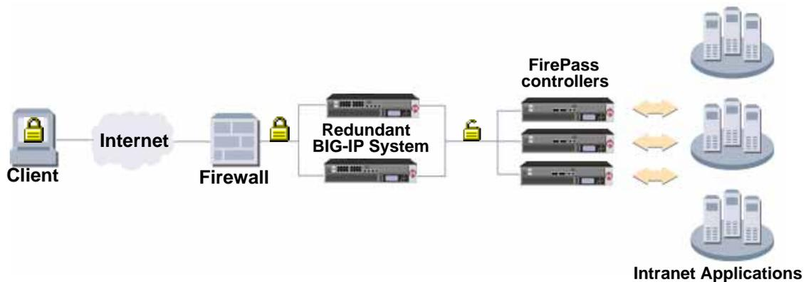
*Figure 1.1 Example BIG-IP/FirePass deployment scenario*
