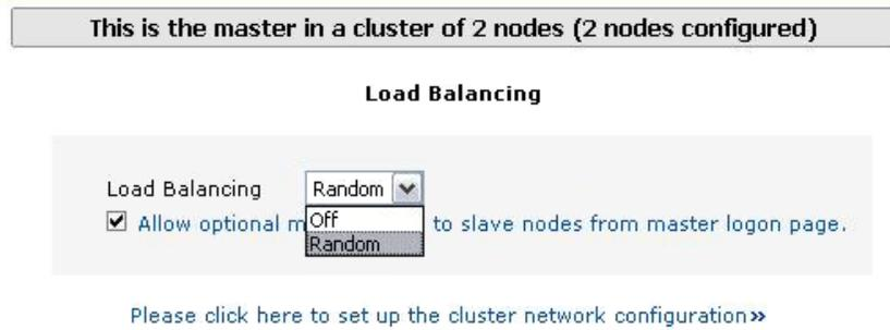
*Figure 1.2 Turning off load balancing on the FirePass controller cluster*
