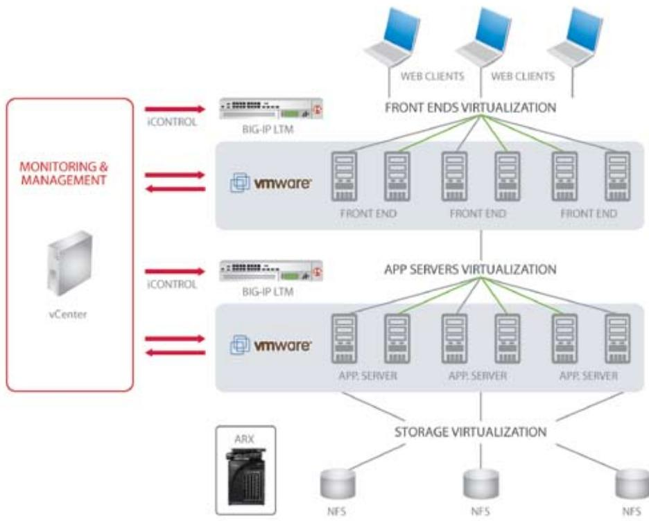
knows when virtual machines or entire data centers are overloaded or unavailable and reroutes traffic accordingly. With its in-built intelligence, BIG-IP can respond to fluctuating traffic loads without the need for manual intervention.
