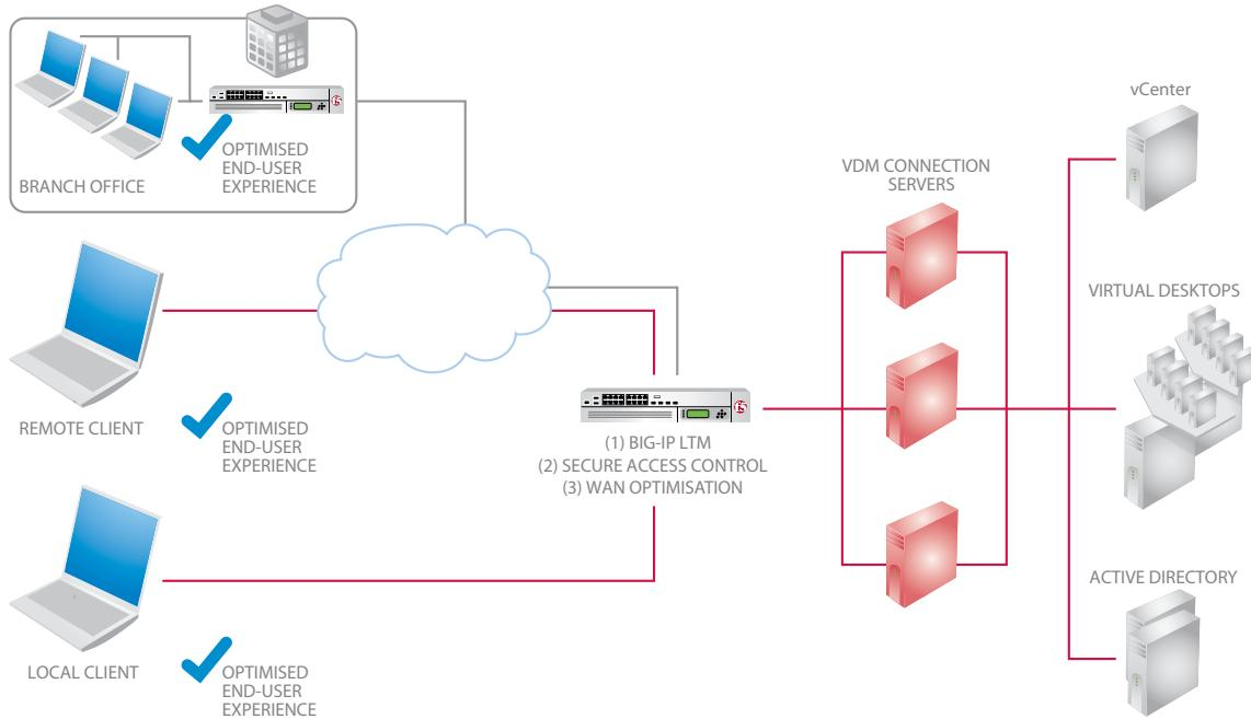
point device prior to allowing the logon sequence to begin, as well as providing a broad range of authentication mechanisms, including two-factor schemes and various back-end directory services. This solution also enforces Active Directory Group policies on any remote device and improves availability.
