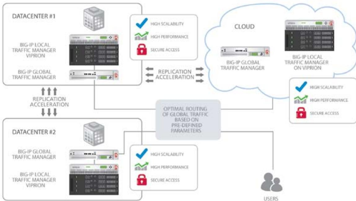
and flexible choice. It provides true network traffic management capacity on demand by allowing additional blades to be added without any manual configuration or interruption in application performance. VIPRION is ideal for service providers as it offers a multitenancy feature that allows administrators to easily slice up VIPRION capacity to manage different customers' traffic separately on a single VIPRION unit.
