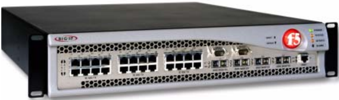
Figure 1.3 An example of a 5000 series IP Application Switch, in this case a BIG-IP 5000
