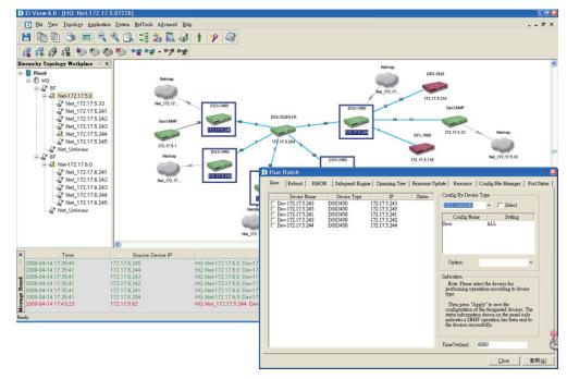
The screens represent D-View 6.0's Batch Configuration feature and its ability to configure multiple devices at a time.
