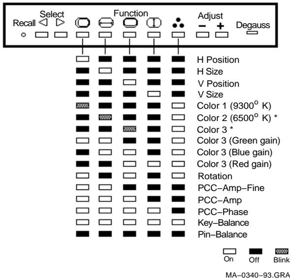
2. When the indicator above the function symbol lights up, the control is active and can be adjusted. Press the  or  buttons to decrease or increase the adjustment. The monitor automatically memorizes all adjustments.
