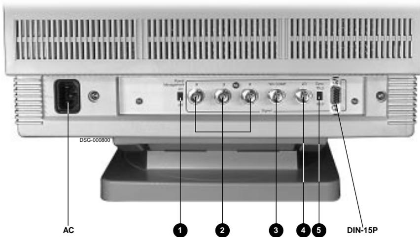
6. Ensure that the Sync switch **5** is set at  $75\Omega$ . (The  $1k\Omega$  position is for TTL sync signals on DIN-15P, which is not supported.)
