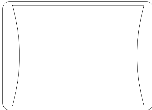
Figure 4-18 Video Area on Screen Bowed Out
