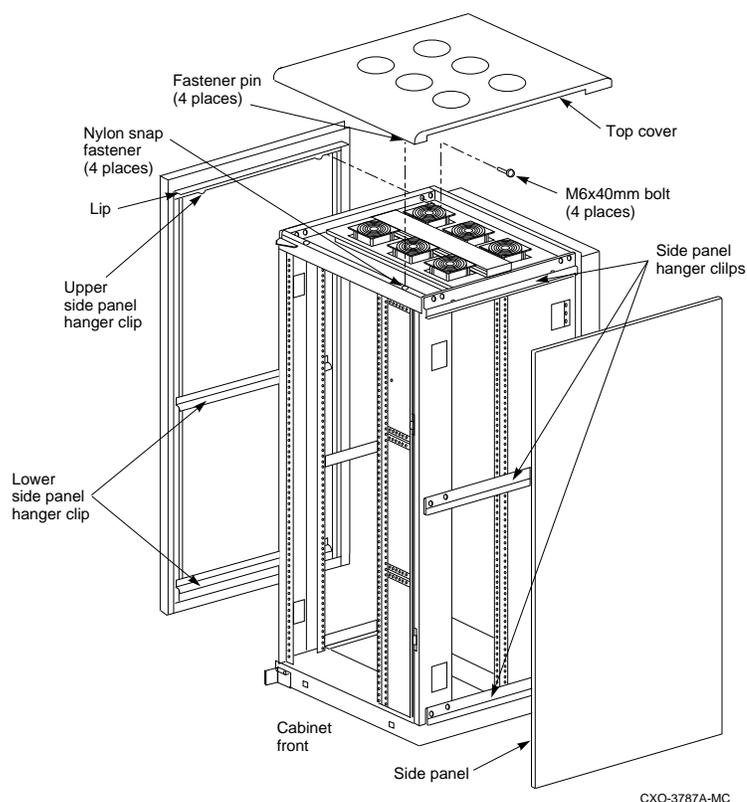
2. Remove the 4 bolts attaching the 2 side panels to the top cabinet side rails.
