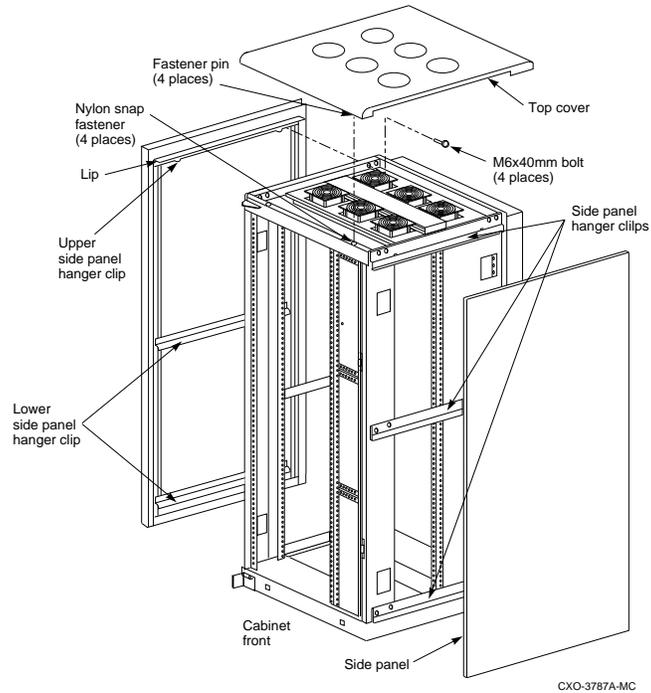
2. Grasp a side panel by the front and rear edges and lift it up so that side panel lip is above cabinet upper side panel hanger clip.
