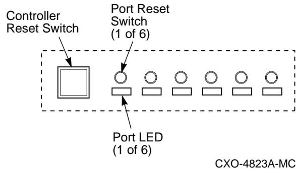
The green controller reset LED indicates controller status. This LED flashes constantly once the controller initialization is complete and the firmware is functioning. Pressing this switch resets the controller.
