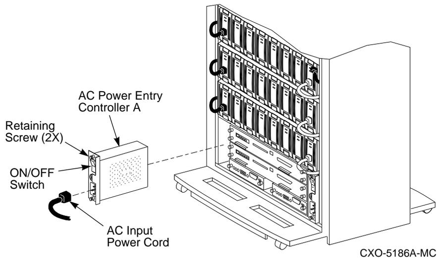
Use the following procedure to install a power entry controller:
