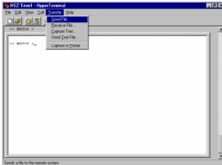
9. Type the location of the firmware image file (V31Z.IMG) in the Filename box. Select *Kermit* in the Protocol box and click the *Send* button.
