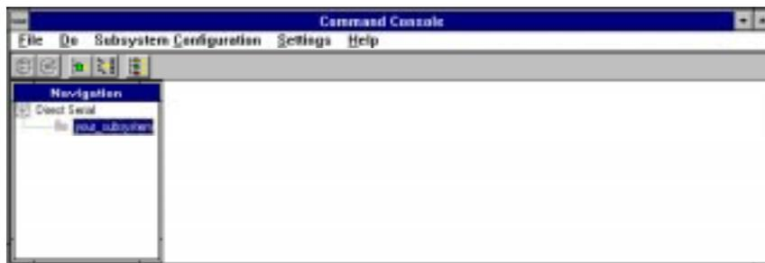
A Divider Bar splits the Control Panel into two smaller windows: the Navigation Window (on the left) and the Subsystem Window (on the right). The Subsystem Window lets you view, configure and monitor the storage subsystem shown in the Navigation Window. The Control Panel also has a Menu Bar and below it a Toolbar. For more information on Command Console’s windows, menus, and tools, refer to the *Command Console User’s Guide*.
