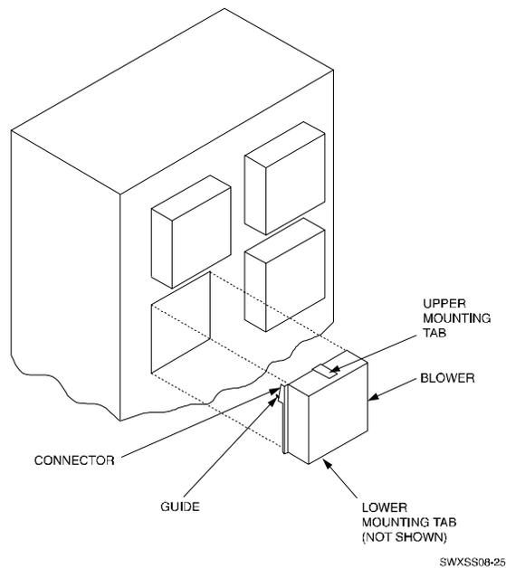
To replace a dual-speed blower, refer to Figure 4–2 and complete the following procedure:
