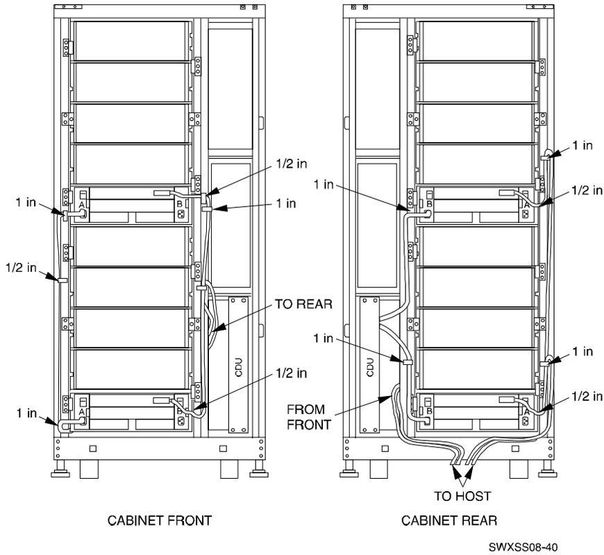
2. Route the power cord through a one-inch cable clamp (fits loosely) on the cabinet vertical rail. You must have at least 16 inches of power cord slack to route from the one-inch clamp to the ac power controller connector.
