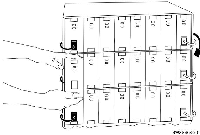
Use the following procedure to install a power supply SBB:
