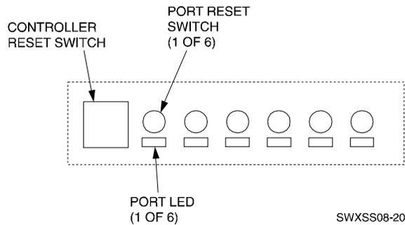
The green controller reset LED indicates the controller and the host interface status. This LED flashes constantly once the controller initialization is complete and the firmware is functioning. Pressing this switch resets the controller.
