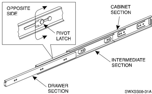
Pivot the latch between the drawer section and the intermediate section to remove the drawer section. Proceed as follows to install the slide drawer section onto a RAID shelf:
